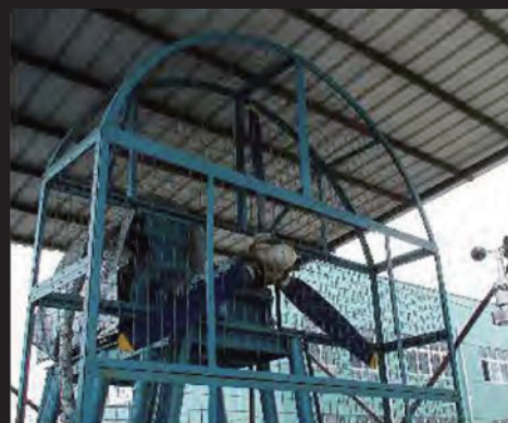
Air Craft Engine (Capable of Producing A Wind Velocity In 50m/s) —Dynamic Water Permeability Test 幕墙动风压装置 (最大风速 50m/s)
